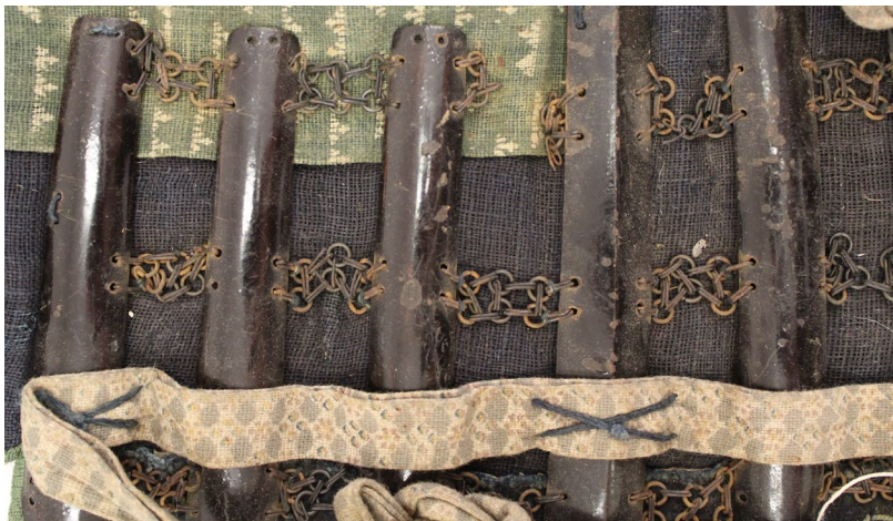
Figure 1: Orange iron corrosion on chain mail.
